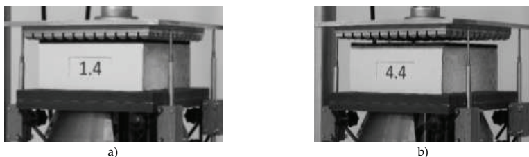
Fig. 1. Examples of tested USP samples attached to concrete blocks: a) sample no. 001; b) sample no. 004 [source: authors' own photos].
