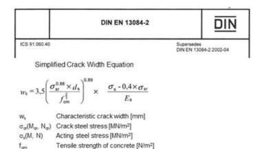
Fig. 3.4: METHOD, Simplified Crack Width in EN 13084, CICIND Model Code, DIN 1056 Crack prediction method gained from the Continuous Deformation Theory
