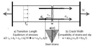
Fig. 3.1: METHOD, Basic crack width equation, a) Transition length a, b) Crack width w
