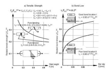
Fig. 2.3: BASES, Crucial material featuresa) Tensile strength of concrete fct, b) Bond low □v(d)
