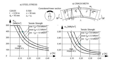
Fig. 5.2.2: APPLIANCE, Windshield of a PP chimney , Impact of reinforcement  $\rho$  and tensile strength  $f_{ct}$ a) Steel Stress  $\sigma_s$  b) Crack width w
