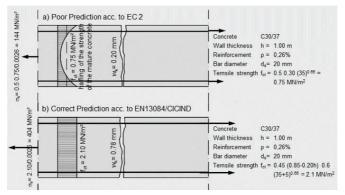
Fig. 5.1.3: APPLIANCE, Bottom Slab in an Underground Parking Lot a) Poor crack prediction acc. to EC2, b) Correct crack prediction acc. to EN 13084/CICIND
