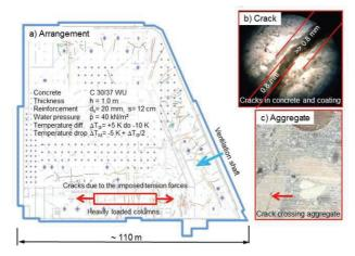
Fig. 5.1.2: APPLIANCE, Bottom Slab in an Underground Parking Lot a) Crack locations, b) Crack in concrete and coating, c) Crack crossing aggregate
