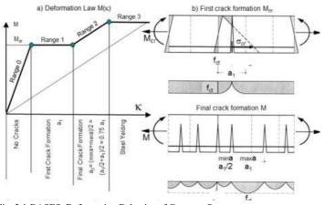
Fig. 2.1:BASES, Deformation Behavior of Concrete Structures Crack formation and transformation of the transition length a1 into the final crack spacing  $a_2$
