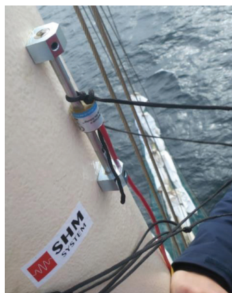
Fig. 3. STS Fryderyk Chopin side view with location of sensors in the first (circle) and the second (triangles) measurements series. Installation of vibrating wire strain gauges [12] [13].
