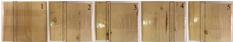
Fig. 9. Double lap shear samples after the test
