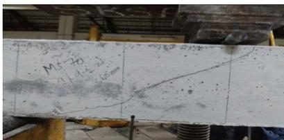
Figure 13: Failure pattern of SFSCC70
