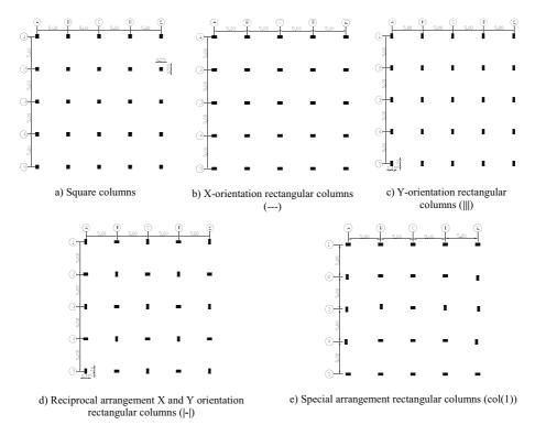
Fig. 1. Square floor plan models with different column orientations and arrangements
