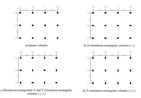
Fig. 2. Rectangular floor plan (ratio 1.5) models with different column arrangements and orientations
