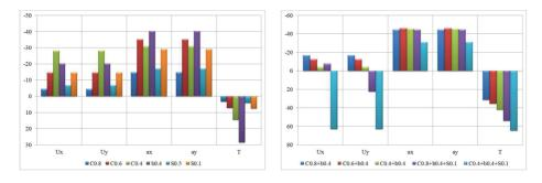
Fig. 4. Percentage ratios of displacement, acceleration, and first mode time period for the square building with square column cross sections
