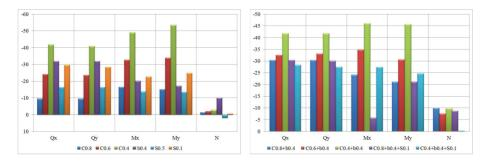
Fig. 5. Percentage ratios of base shear force, base bending moment, and base normal force for the square building with square column cross sections
