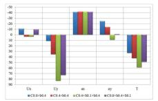
Fig. 7. Percentage ratios of displacement, acceleration, and first mode time period for the rectangular (ratio 2.5) building with square column cross sections
