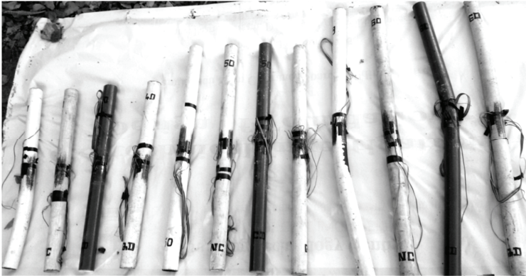
Fig. 3. Tested concrete filled tubular columns
