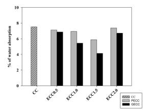
Fig 6. Results showing % of water absorption after 28 days of water curing
