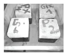
Fig 7. Sorptivity test specimen
