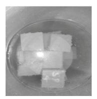
Fig 1. Specimen immersed in water diluted with 5% sodium sulphate powder
