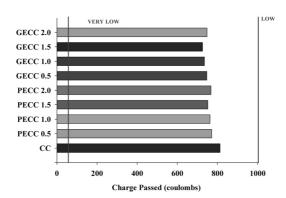
Fig 10. RCPT values of various mixes of ECC
