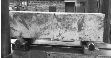
Fig. 2. Experimental test of beam element 100x100x400mm
