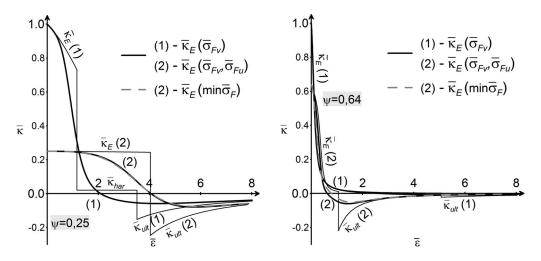
Fig. 7. Comparison of deterministic and probabilistic tangent axial stiffness of eccentrically connected brace corresponding to force-deformation characteristics from Figure 6; a) stocky angle  $\overline{\lambda}_{Fv} = 0,5$ , b) slender angle  $\overline{\lambda}_{Fv} = 2,0$ .
