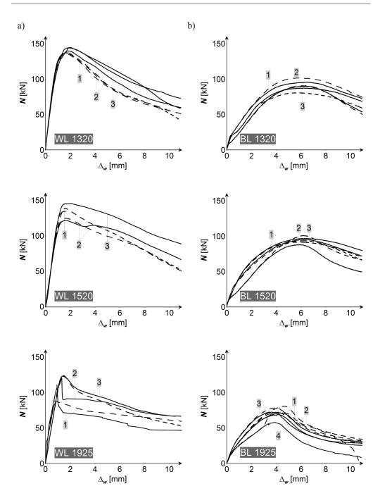
Fig. 12. Experimentally obtained force-deformation characteristics of bracing members, a) frame specimens WL, b) frame specimens BL; 1, 2, 3 and 4 – numbers of specimens [33].
