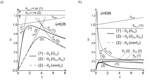
Fig. 6. Comparison of dimensionless deterministic and probabilistic force-deformation characteristics of angle brace using the parameters:  $a_h = 0,02$ ,  $a_u = 1$ , and (1) – in-plane eccentricity for which  $e_u = 10$  mm, n = 5, (2) – space eccentricity for which  $e_u = 2$  mm,  $e_v = 28$  mm, n = 3,5; a) stocky angle  $\overline{\lambda}_{Fv} = 0,5$ , b) slender angle  $\overline{\lambda}_{Fv} = 2,0$ .
