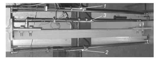
Fig. 10. Details of brace shortening measurement using LVDT devices mounted to a specimen of BL group; 1, 2 and 3 – LVDT devices [33].
