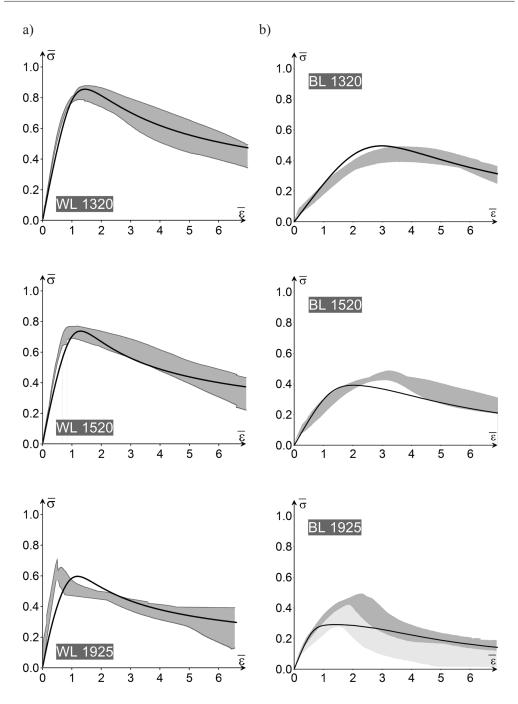
Fig. 13. Comparison of analytical force-deformation characteristic with experimental envelope of results: a) WL type braces, b) BL type braces.
