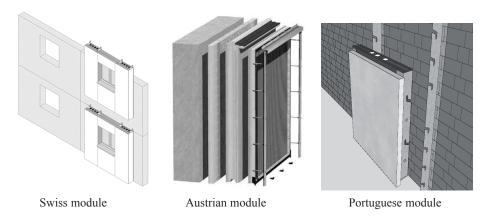
Fig. 1. Examples of prefab modules developed by IEA ECBCS Annex 50 project [22]
