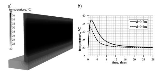
Fig. 4. Distribution of temperature in the wall: a) map of thermal fields (¼ of the L\_28,d\_0.7 wall) at the moment of reaching the maximum hardening temperature, b) diagram of temperature development in time – the centre section for the L\_28 wall with 0.7 m and 0.4 m thickness.
