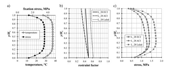
Fig. 6. The case of non-uniform distribution of temperature – wall L\_28,d\_0.7: a) distribution of temperature at the height of the wall (at the moment of reaching the maximum hardening temperature) and fixation thermal stress, b) restrain factor at the height, c) total thermal stress at the height after 28 days.
