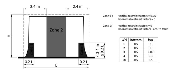
Fig. 2. Axial restraint factor  $R_{ax}$  in element restrain along one edge [4].
