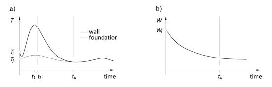
Fig. 1. Temperature (a) and moisture content (b) development in time for an externally restrained concrete wall [7].
