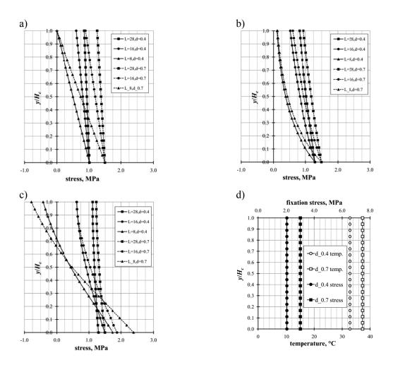
Fig. 5. The case of uniform distribution of temperature: distribution of total thermal stress in centre crosssection of the walls according to EC2 (a), ACI (b) and Luleå (c) method, d) assumed uniform temperature at the height of the wall (at the moment of reaching the maximum hardening temperature) and fixation stress distribution for the walls with 0.4 m and 0.7 m thickness.
