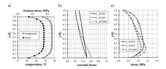
Fig. 7. The case of non-uniform distribution of temperature – wall L\_16,d\_0.7: a) distribution of temperature at the height of the wall (at the moment of reaching the maximum hardening temperature) and fixation thermal stress, b) restrain factor at the height, c) total thermal stress at the height after 28 days
