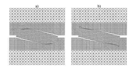
Fig. 21. Nooru-Mohamed [33] test: calculated cracks for different averaging length l: (Eq. 3.4): a) l = 0.5 mm and b) l = 2 mm (crack model by Cox [26]).
