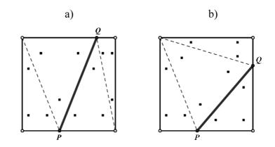
Fig. 4. Integration schemes in 4-node quadrilaterals: a) divided into 2 quadrilaterals and b) divided into trapezoid and triangle.
