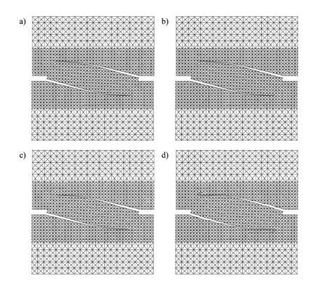
Fig. 22. Nooru-Mohamed [33] test: calculated cracks for different relative minimum distances from element vertices: a) 1%, b) 2%, c) 10% and d) 20% (crack model by Cox [26]).
