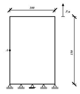
Fig. 5. Uniaxial tension numerical test: geometry and boundary conditions (P – vertical force along upper edge, u – vertical displacement of upper edge, A – crack start point).
