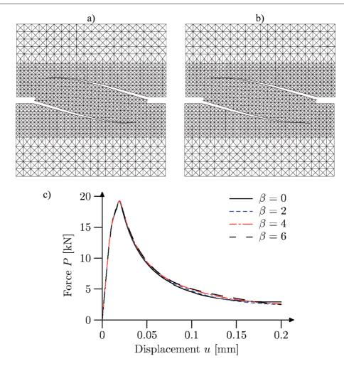
Fig. 20. Nooru-Mohamed [33] test: calculated cracks with coupling parameter  $\beta$  (a)  $\beta$  =0 and b)  $\beta$  =4) and force-displacement curves c) (model by Unger et al. [27]).
