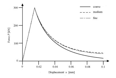
Fig. 6. Uniaxial tension numerical test: force-displacement diagrams for different FE meshes.
