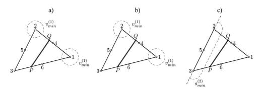
Fig. 2. Minimum distances between crack segments and triangle vertices/sides: a)  $v_{\min}$ , b)  $l_{\min}$  and c)  $s_{\min}$ .
