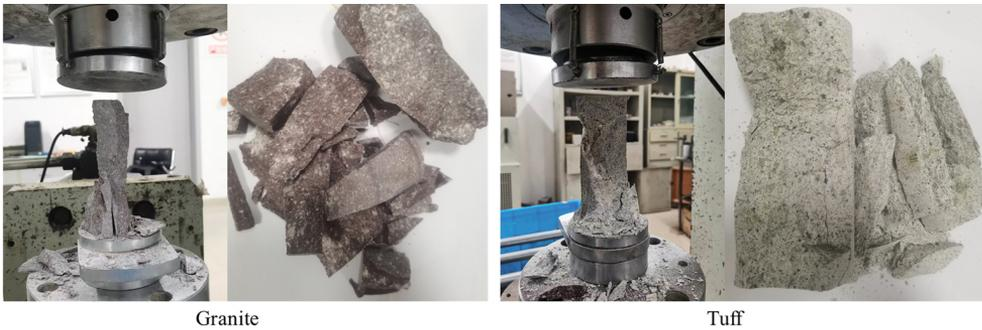
Fig. 8. Macro-damage failure states of granite and tuff under uniaxial compression
