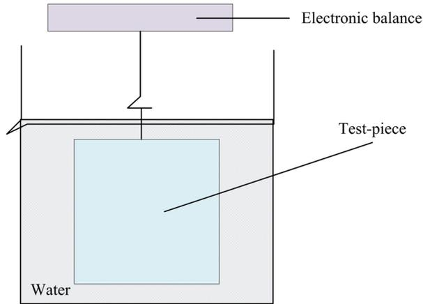
Fig. 2. Schematic diagram of water testing of specimens
