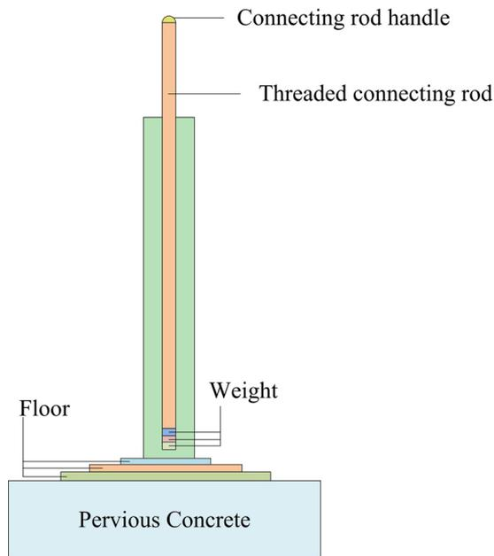
Fig. 1. Improved drop hammer device for modified PC
