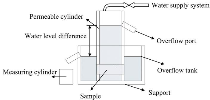
Fig. 3. Schematic diagram of permeability coefficient test device
