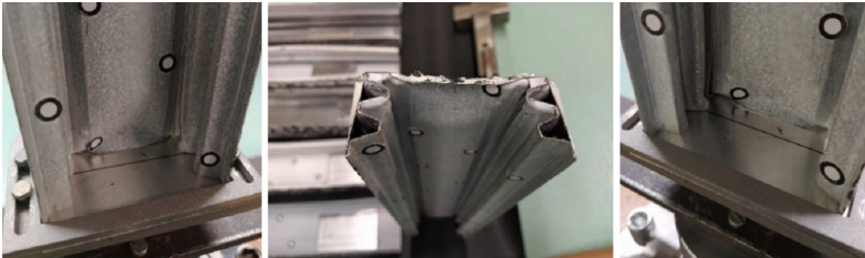
Fig. 8. Columns after performed tests
