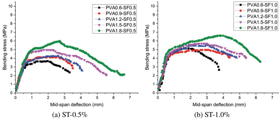
Fig. 10. Flexural stresses versus midspan deflection curves of beams with 50% ceramic powder
