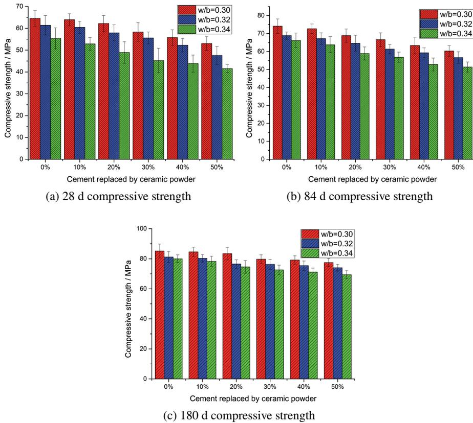
Fig. 6. The compressive strength of mortar contains ceramic wastes
