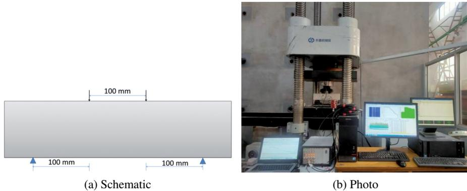
Fig. 7. Loading of a beam
