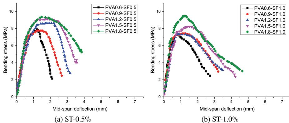
Fig. 8. Flexural stresses versus midspan deflection curves of beams with 0% ceramic powder
