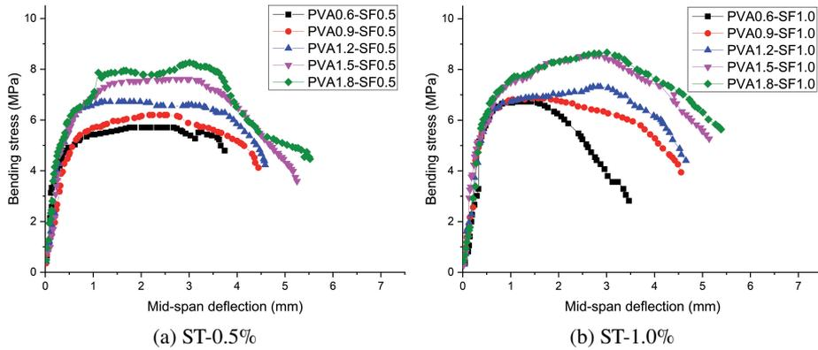
Fig. 9. Flexural stresses versus midspan deflection curves of beams with 30% ceramic powder
