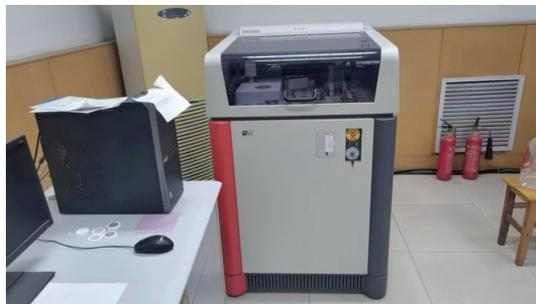
Fig. 3. X-Ray Fluorescence Spectroscopy tester(BRUKER S4 Explorer)
