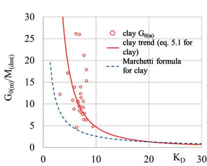
Fig. 5. Relationships between ratio  $\frac{G_{0(m)}}{M_{DMT}}$  and  $K_D$  index for clay
