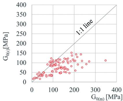
Fig. 16. Relationships between measured shear modulus  $G_{0(m)}$  and calculated shear modulus  $G_{0(c)}$  after Marchetti equation for sand
