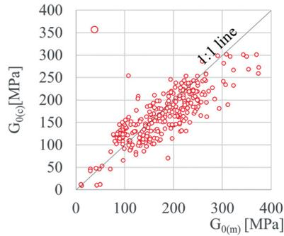
Fig. 8. Relationships between measured shear modulus  $G_{0(m)}$  and calculated shear modulus  $G_{0(c)}$  after Marchetti equation for sandy loam
