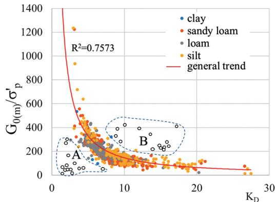
Fig. 17. Relationships between measured shear modulus  $G_{0(m)}$  normalized by  $\sigma'_p$  and  $K_D$  parameter for clay, sandy loam, loam and silt
