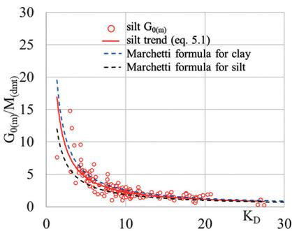
Fig. 11. Relationships between ratio  $\frac{G_{0(m)}}{M_{DMT}}$  and  $K_D$  index for silt
