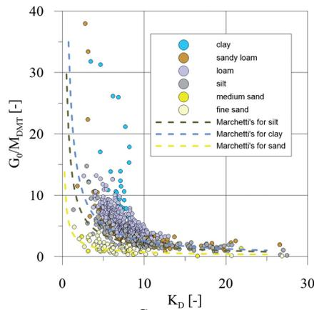
Fig. 4. Relationship between ratio  $\frac{G_{0(m)}}{M_{DMT}}$  and  $K_D$  index for investigated soils on the background of original Marchetti et al. [1] formulas
