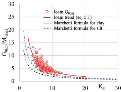
Fig. 9. Relationships between ratio  $\frac{G_{0(m)}}{M_{DMT}}$  and  $K_D$  index for loam
