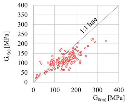
Fig. 12. Relationships between measured shear modulus  $G_{0(m)}$  and calculated shear modulus  $G_{0(c)}$  after Marchetti equation for silt
