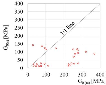
Fig. 6. Relationships between measured shear modulus  $G_{0(m)}$  and calculated shear modulus  $G_{0(c)}$  after Marchetti equation for clay
