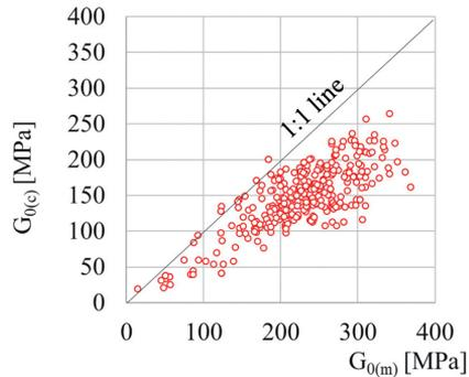
Fig. 10. Relationships between measured shear modulus  $G_{0(m)}$  and calculated shear modulus  $G_{0(c)}$  after Marchetti equation for loam
