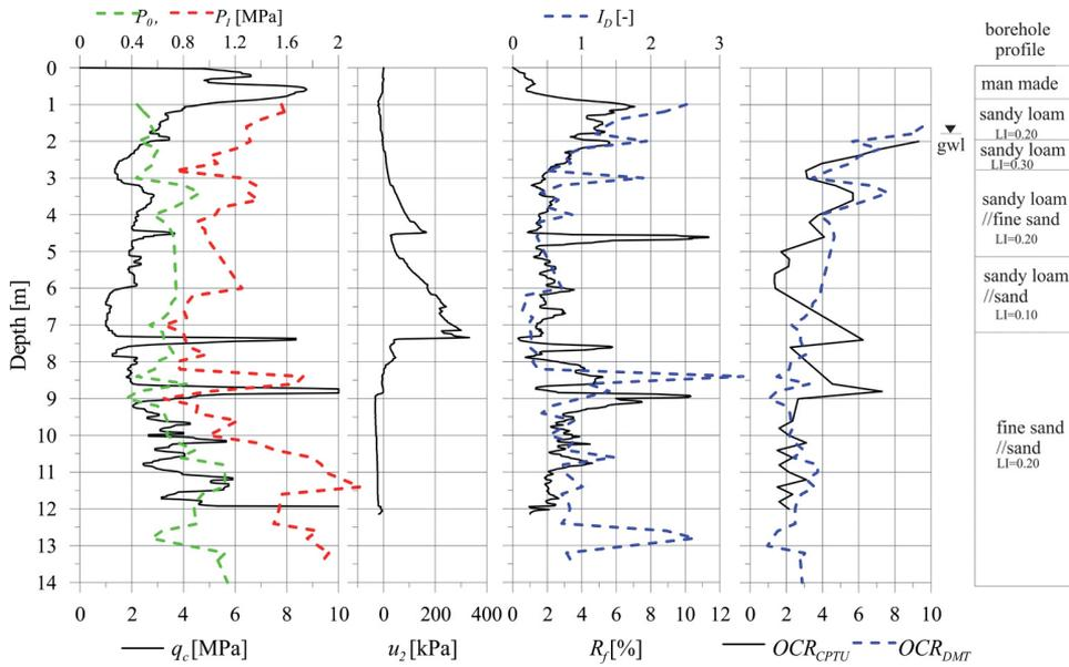
Fig. 2. CPTU, DMT and borehole profile with calculated OCR profile at Lipno test site
