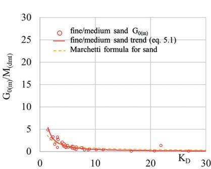
Fig. 13. Relationships between ratio  $\frac{G_{0(m)}}{M_{DMT}}$  and  $K_D$  index for fine/medium sand
