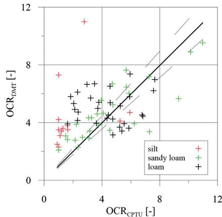
Fig. 3. Comparison of OCR calculated on the basis of CPTU and DMT at Łańcut (silt), Jarocin (loam) and Lipno (sandy loam) test sites with 95% confidence intervals for 1:1 line
