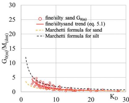
Fig. 15. Relationships between ratio  $\frac{G_{0(m)}}{M_{DMT}}$  and  $K_D$  index for fine/silty sand
