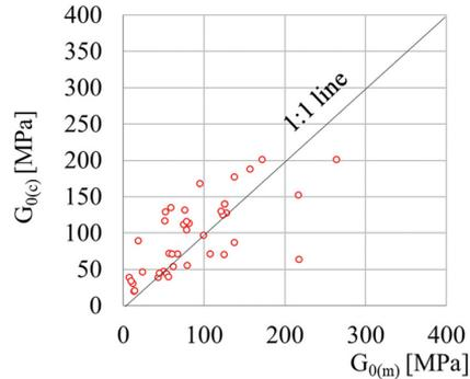
Fig. 14. Relationships between measured shear modulus  $G_{0(m)}$  and calculated shear modulus  $G_{0(c)}$  after Marchetti equation for sand
