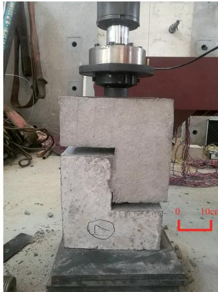
Fig. 3. Shear test set-up
