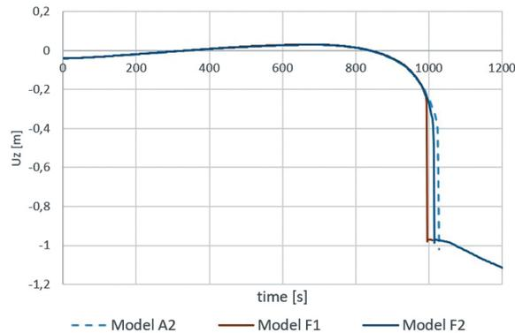
Fig. 17. Estimates of fire resistance for transverse frame exposed to fire action obtained after application of models F1 and F2 juxtaposed with analogous estimate obtained for model A2. Static equilibrium paths refer to the vertical displacement in ridge
