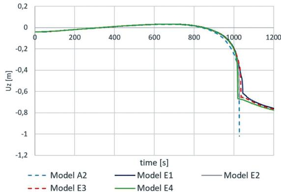
Fig. 15. Fire resistance estimates for a transverse frame exposed to fire actions obtained after application of models E1, E2, E3 and E4 juxtaposed with analogous estimate obtained for model A2. Static equilibrium paths pertain to the vertical displacement at ridge
