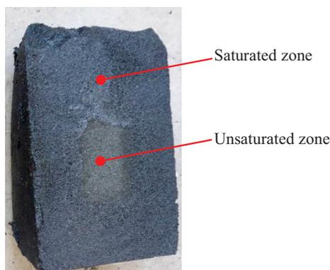
Fig. 4. Cross-section through an saturated foam glass specimen
