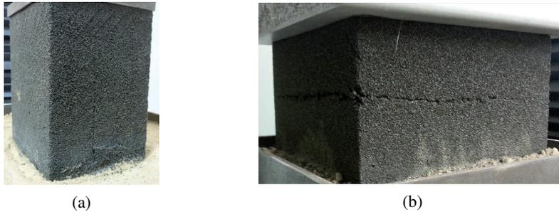
Fig. 10. Example of samples during the tests: (a) vertical fracture, (b) horizontal fracture
