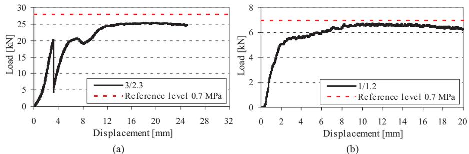
Fig. 5. Load-displacement diagram: (a) specimen 3/2.3 200 × 200 mm – horizontal fracture mode, (b) specimen 1/1.2 100 × 100 mm – gradual crushing mode
