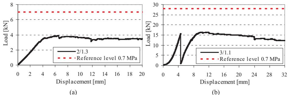
Fig. 9. Load-displacement diagram: (a) specimen 2/1.3  $100 \times 100$  mm – vertical fracture mode, (b) specimen 3/1.1  $200 \times 200$  mm – sudden horizontal fracture mode
