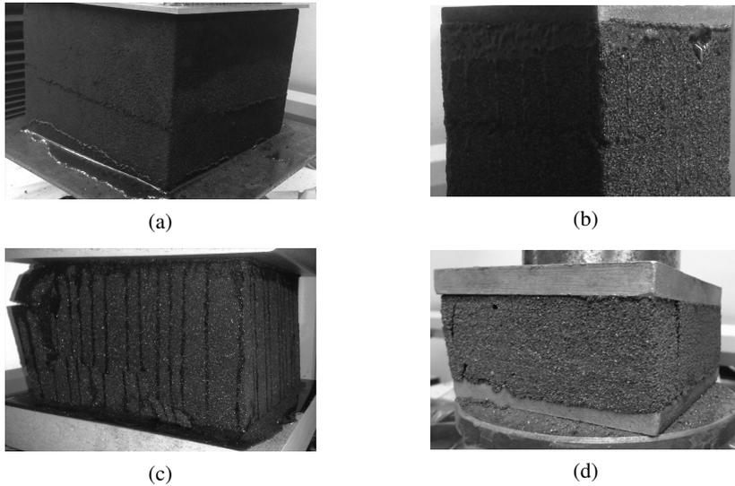
Fig. 6. Example of samples during the tests: (a) horizontal fracture, (b) crushing in the pressure zone and horizontal fracture, (c) crushing in the pressure zone and splitting, (d) fracture in different planes
