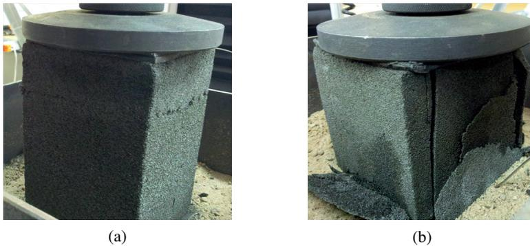
Fig. 12. Specimens during the tests: (a) horizontal fracture, (b) oblique and vertical fracture
