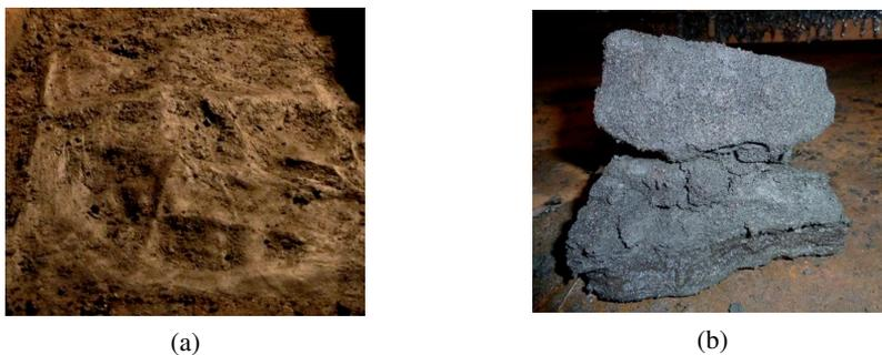
Fig. 3. Surface undulations of the lower foam glass layer (a) and foam glass deterioration (b)
