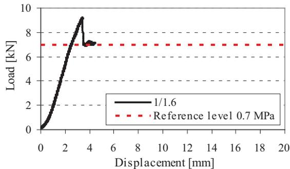
Fig. 7. Load-displacement diagram for vertical fracture mode – specimen 1/1.6 100 × 100 mm
