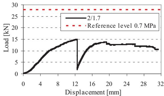
Fig. 11. Load-displacement diagram for the sudden horizontal fracture mode
