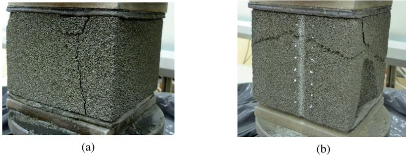
Fig. 8. Example of samples during the tests: (a) vertical fracture, (b) horizontal fracture
