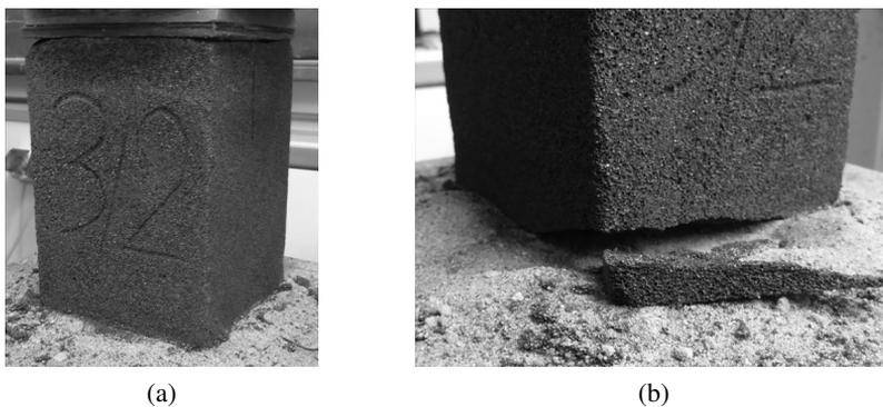
Fig. 13. A sample during the tests: (a) initial phase, (b) chipping in the bottom part of the specimen
