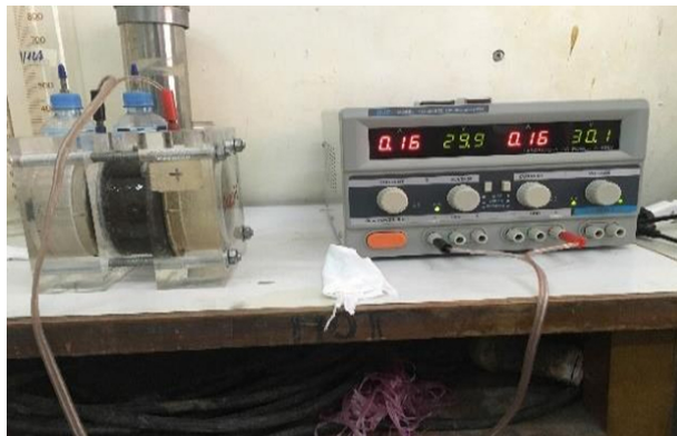
Fig. 6. Chloride ion penetration test
