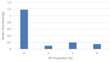
Fig. 6. Binder drain down vs Nano Titanium
