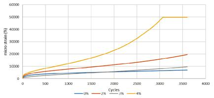
Fig. 3. Strain Values for each modified SMA Specimen
