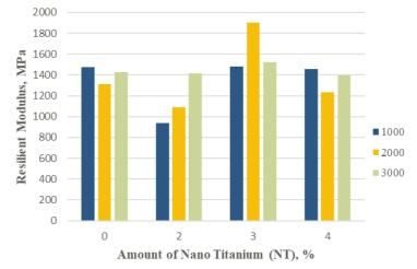
Fig. 1. Resilient modulus of Asphalt Mixtures at Different Dosages of Nano Titanium at 25°C
