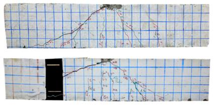
Fig. 4. Cracking failure mode of NB-16 (top) and RB-16 (bottom)
