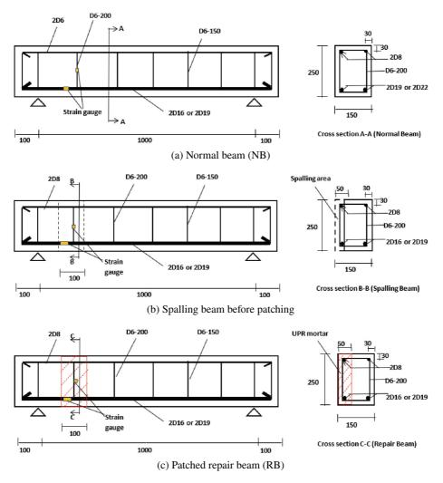
Fig. 2. Beam specimens and their reinforcements lay out
