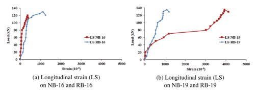
Fig. 6. Load-longitudinal strain behavior of normal and repair beams
