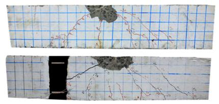
Fig. 5. Cracking failure mode of NB-19 (top) and RB-19 (bottom)
