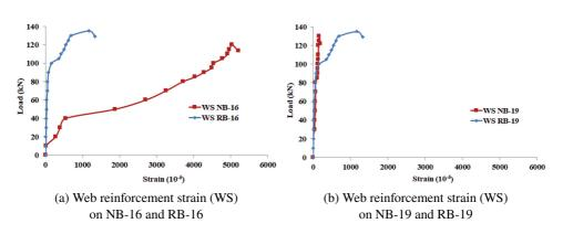
Fig. 7. Load-web reinforcement strain behavior of normal and repair beams
