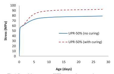
Fig. 1. Strength improvement of UPR mortar when exposed to water
