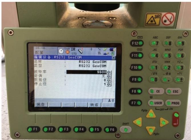
Fig. 4. The serial port of total station
