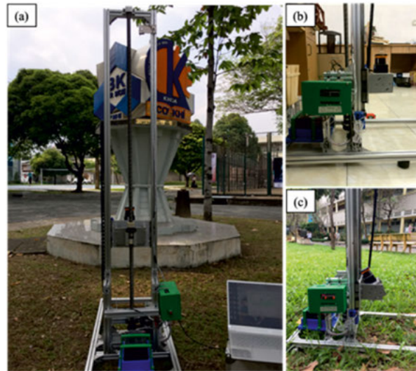
Fig. 3. Data acquisition at one viewpoint. (a) The device moves along the rail from the bottom to capture the image of the object. (b) Illustration nadir and (c) oblique scanning
