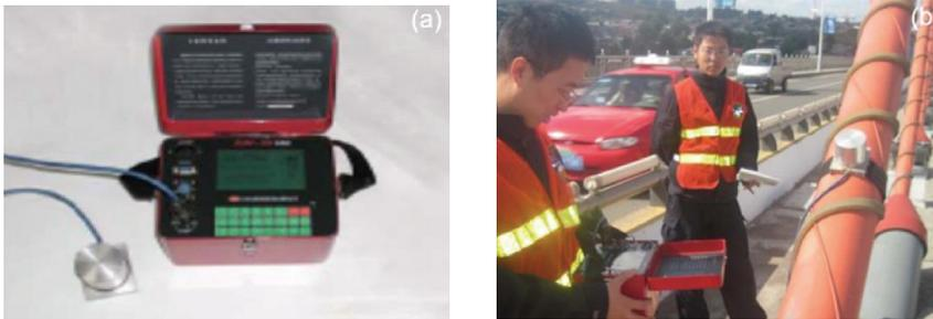
Fig. 5. Test system for cable force
