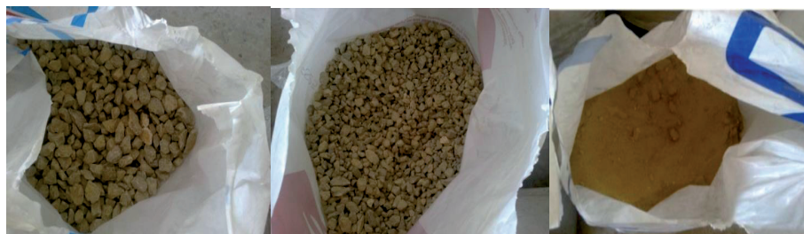
Fig 1. The types of coarse and fine aggregates employed in the experiment
