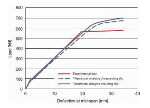
Fig. 12. Results of theoretical analyses vs. experimental tests for beam BZ-6.
