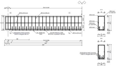
Fig. 3. Dimensions and reinforcement of beams.
