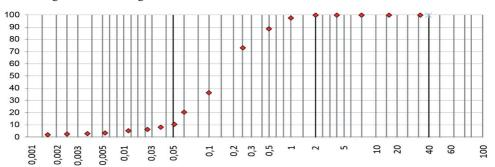
Fig. 1. Granulation curve of the tested soil.
