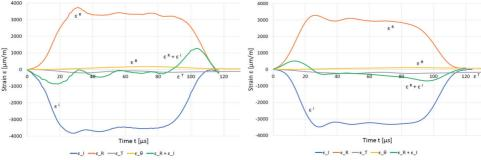
Fig. 8. List of dependencies of longitudinal strain of the bars  $(\varepsilon^I, \varepsilon^R, \varepsilon^T)$  and the peripheral strain of the casing  $\varepsilon^\theta$  depending on the time t - sample  $w_1 = 0$  [%].
