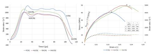
Fig. 14. A collective list of soil strain rate charts  $\dot{\varepsilon}$  over time t.
