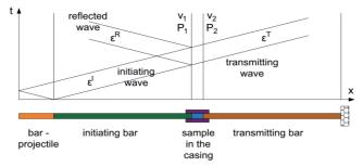
Fig 4. Wave chart illustrating the phenomenon of elastic wave propagation in a Split Hopkinson Pressure Bar. t - time, x - bar axis: bar-projectile and measuring bar,  $\varepsilon^I(t)$ ,  $\varepsilon^R(t)$  - elastic strain of the measuring bars over time measured by strain gauges,  $P_1(t)$  and  $P_2(t)$  - dynamic forces at the ends of the tested sample,  $v_1(t)$  and  $v_2(t)$  - the velocity of the fronts of the measuring bars.
