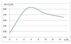
Fig. 18. Change in the content of fine fractions in the soil after the next test, depending on the moisture content.
