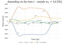
Fig. 11. List of dependencies of longitudinal strain of the bars  $(\varepsilon^I, \varepsilon^R, \varepsilon^T)$  and the peripheral strain of the casing  $\varepsilon^\theta$  depending on the time t - sample  $w_4 = 14.6$  [%].
