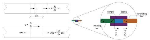
Fig. 6. Diagram of elastic wave propagation in a measuring bar [5].
