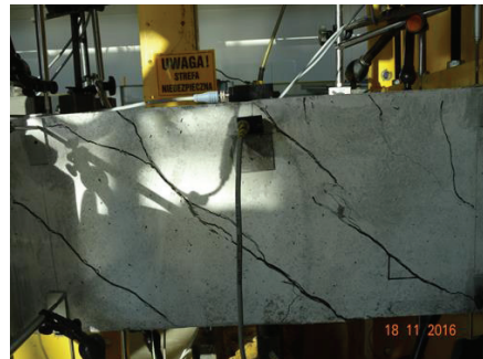
Fig. 5. The cracks image of the analysed beams, a) beam B1, b) beam B3
