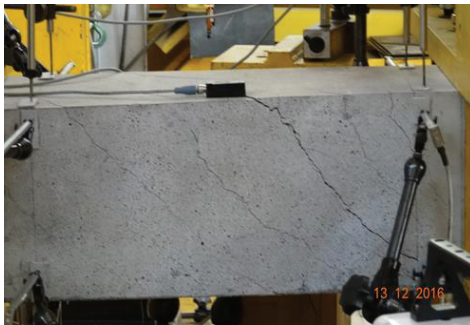
Fig. 5. The cracks image of the analysed beams, a) beam B1, b) beam B3
