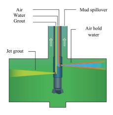
Fig. 4 Triple pipe method of high-pressure jet grouting pile (T-construction method)
