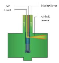
Fig. 3 Double pipe method of high-pressure jet grouting pile (D-construction method)
