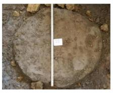
Fig. 7 Pile diameter inspection (up to 900mm)
