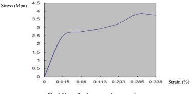
Fig. 9 Unconfined compressive strength test
