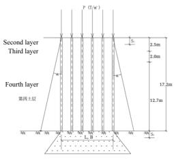
Fig. 12 Schematic Diagram of Foundation Deformation Calculation
