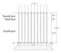
Fig. 11 Schematic Diagram of Foundation Deformation Calculation
