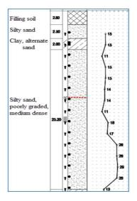
Fig. 6 Schematic Diagram of Typical Geological Axis
