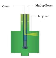
Fig. 2 Single pipe method of high-pressure jet grouting pile (S-construction method)
