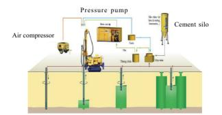
Fig. 1 Schematic diagram of equipment and construction procedure of high pressure jet grouting pile
