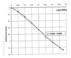
Fig. 10 Field Plate Load Test Results of High Pressure Jet Grouting Pile
